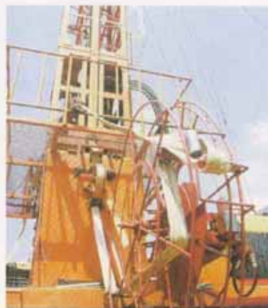
Twist preventive device and back tension reel
